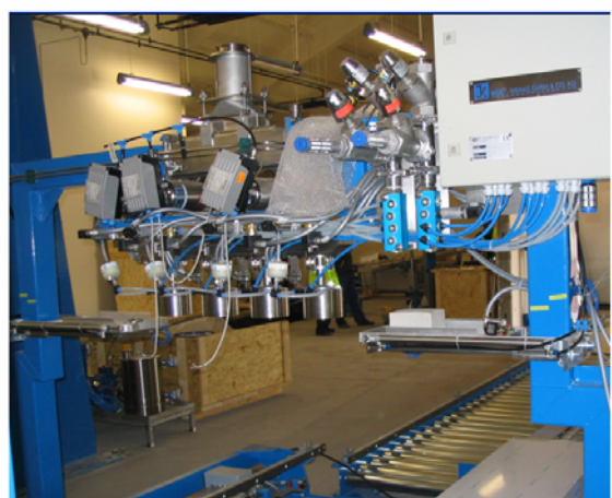
Figure 8 The pallet conveyor and the 4 head filling system
